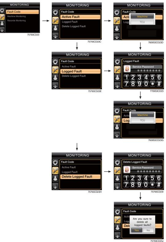
· Monitor the fault code of the Machine/TCU.
