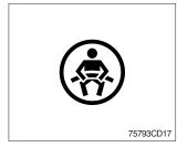
① This lamp lights ON for the first five seconds after starting the engine.
